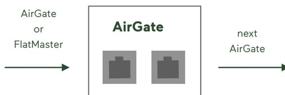
Therefore a pre-fabricated 25 cm (10') cable (RJ12) is included. For other installations the following connection lengths are available: 25, 50 100 and 200 cm (10, 20, 40 and 80').
